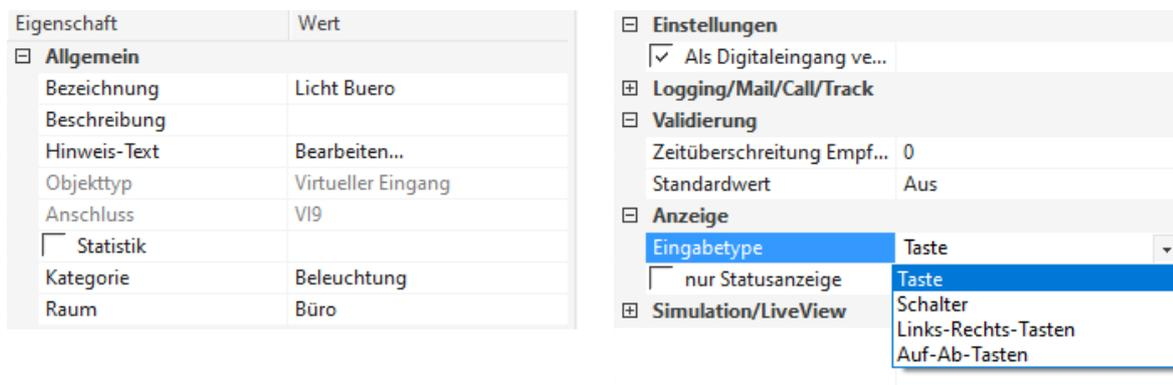
In this case, the URL is called "post://username:passwort@192.168.1.10/dev/sps/io/VI9/pulse", which is called by pressing button 1 in Dingz. In Loxone, an impulse is triggered in VI9.
